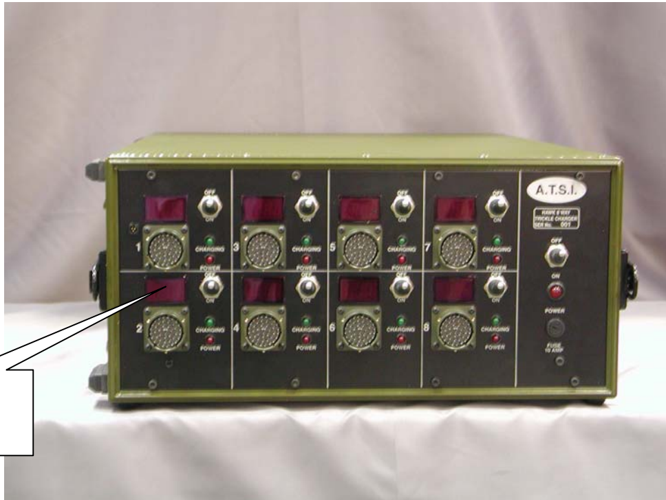
(6) Battery Voltage Meter
